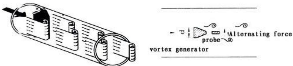
Figure1 The working principle of the vortex-shedding flowmeter
