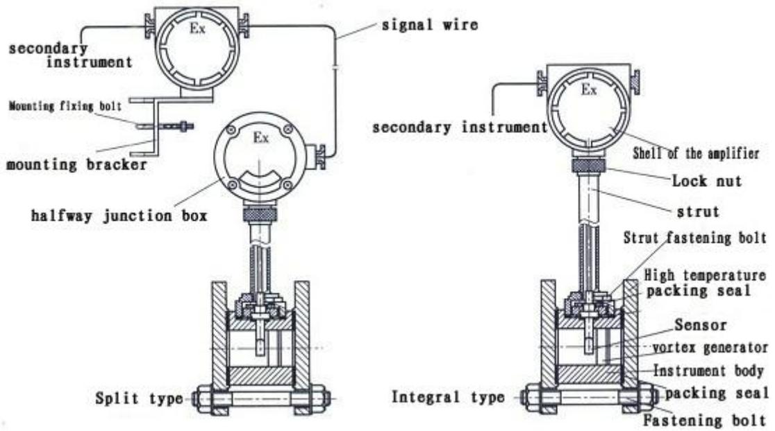
Figure2 The schematic diagram of instrument structure
